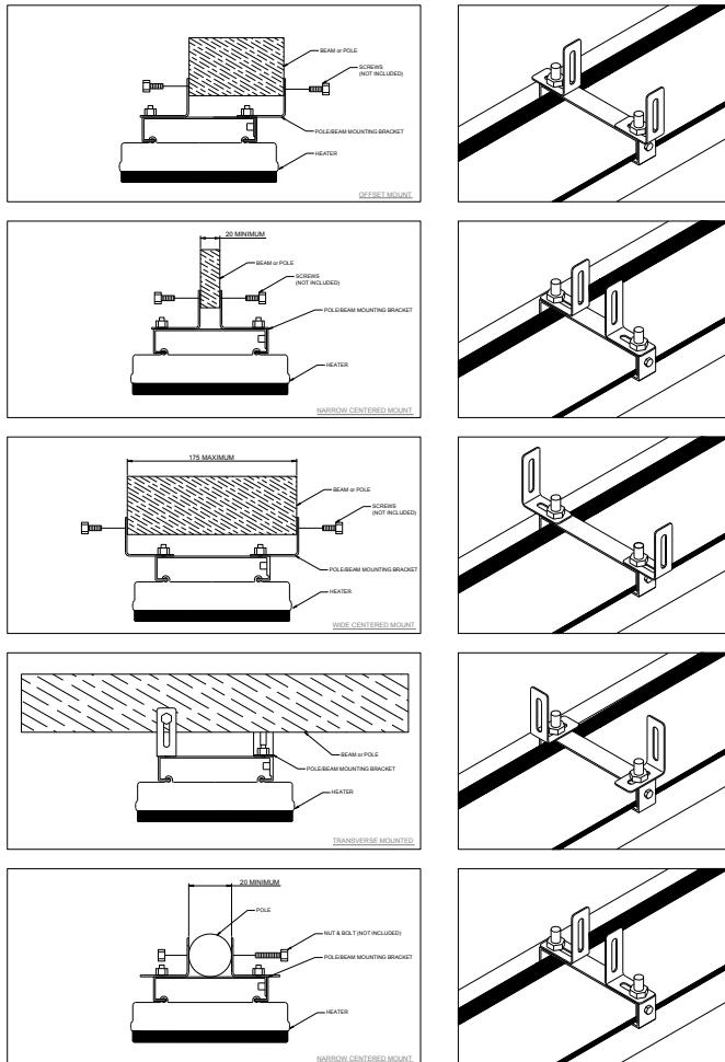
The optional Pole/Beam mounting bracket kit can be used to mount HEATSTRIP Design onto wooden beams, rafters, poles, umbrellas struts etc.
