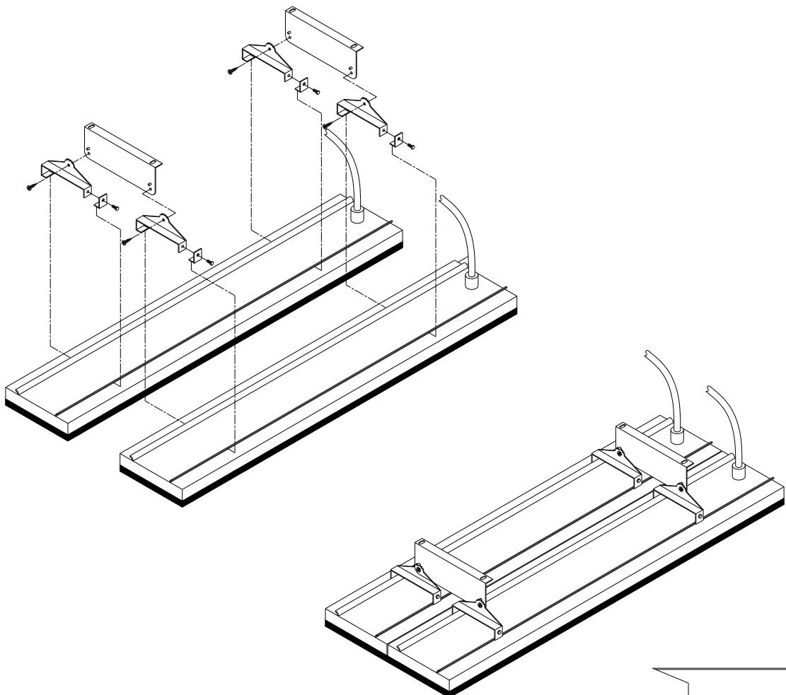
The optional Twin Mount bracket allows for two (2) units of HEATSTRIP Design to be mounted side-by-side, either in parallel or angled as per the diagram on the right. This is ideal for applications when a wider heat coverage is required, or when there is mounting restrictions/limitations (such as running between 2 rows of tables etc.)
