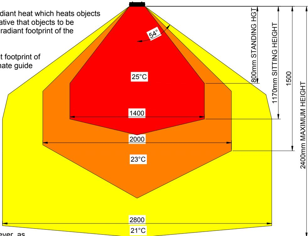
The below diagrams show the approximate heating area for each model, based on both an indoor and outdoor enclosed environment, with direct overhead mounting.
